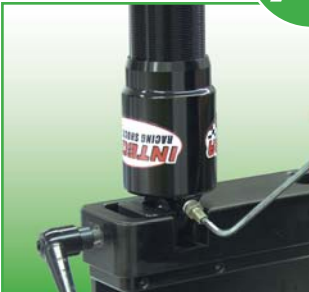
A1 Discharge nitrogen gas prior to disassembly
