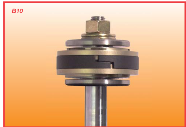
Place piston washer & nut on piston rod
