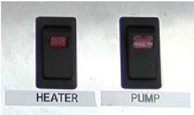
Figure 4: Switches shown in off position.
