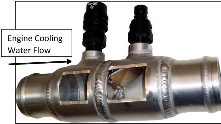
Figure 7: Assembled inline flapper valve cutaway. The valve is open as if during normal engine operation, and the quick connect fittings seal shut.
